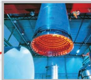
Hot Isostatic Pressing (HIP) ensures that any porosity within the part is removed, thereby reducing the variation in mechanical properties when compared with the as-built part, and improving ductility and fatigue strength.
